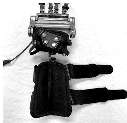
Remove one side of the forearm straps from the D-rings and lay to side.
