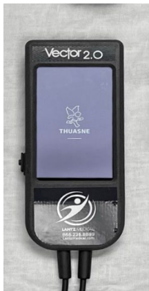
The blue screen rendering the ThuasneUSA logo ensures the unit is properly powered.
