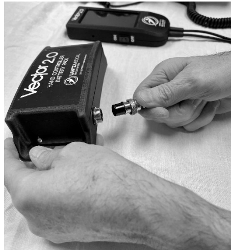
Connect the hand controller to the battery pack, or (see next image.)
